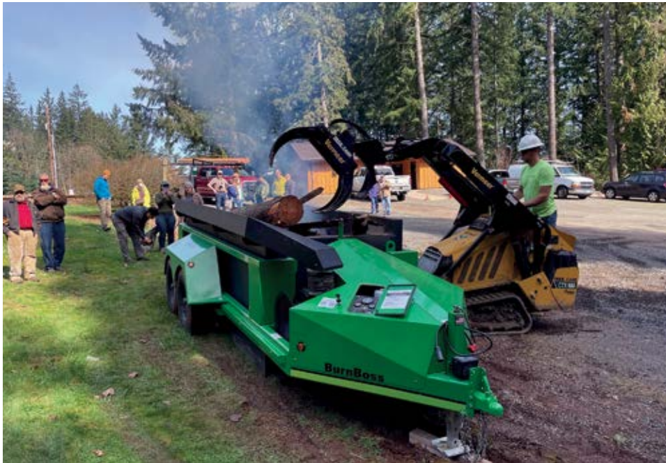
Air curtain burner demonstration at Hopkins, showing a method of debris burning with reduced smoke emissions (March 2022).
